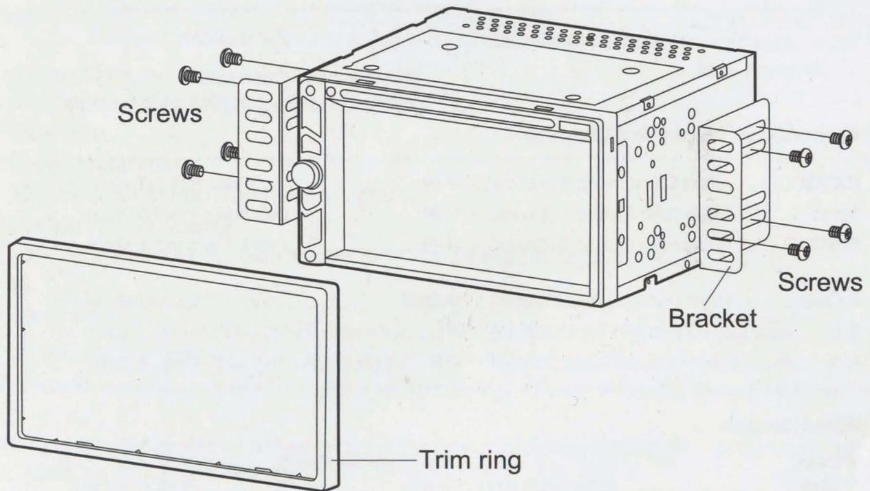
1. Put the 2 brackets to the left and right side of the unit.
